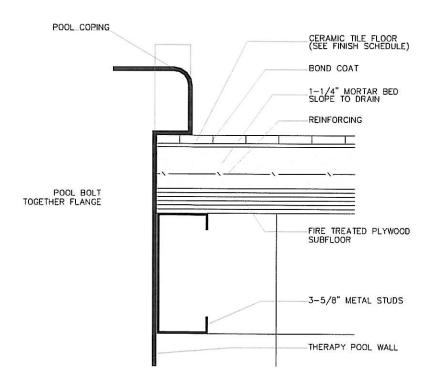
The deck material should slope slightly away from the pool to prevent water from draining into pool.
