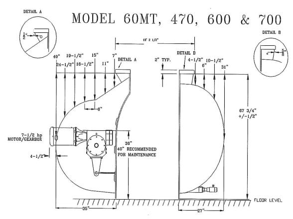
NOTE: The tolerance of +/- 1/2" is due to the compression of the foam pad. ALL OTHERS +/- 1/4"
